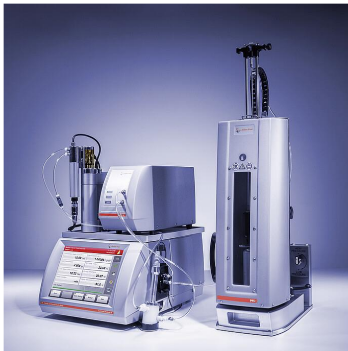
Figura 7 – Equipamento Soft Drink Analyzer (Anton Paar, s.d.)
